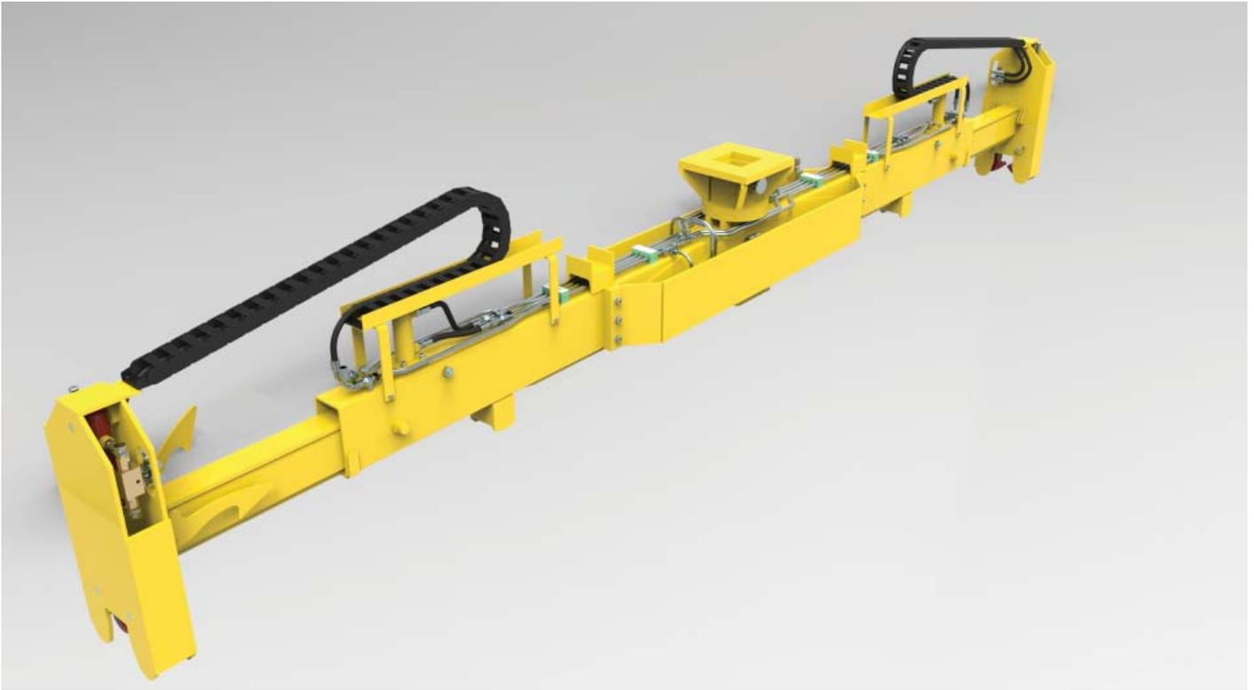
*The TRLB20 fitted with square drive head has a safe working load of 1,250kg and is proof load tested to 2,500kg.*
