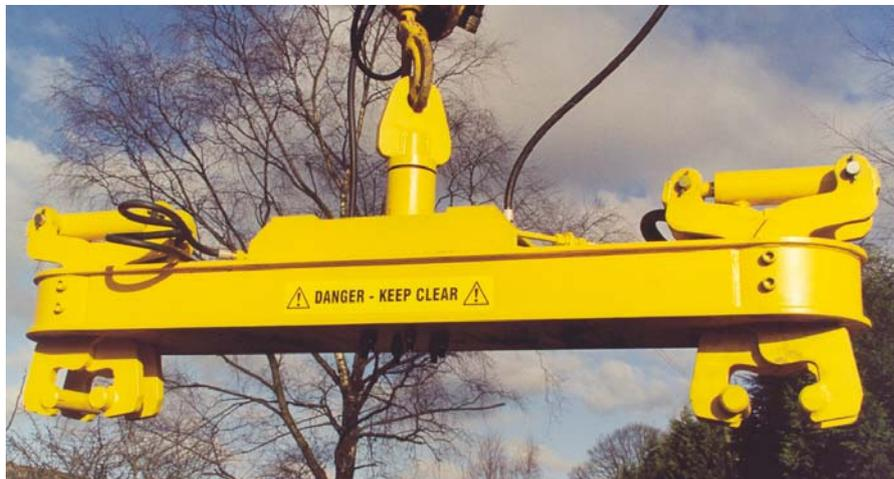
Suspend the beam from a hook, shackle or lifting device suitably rated for the weight of the beam and the imposed load combined.
