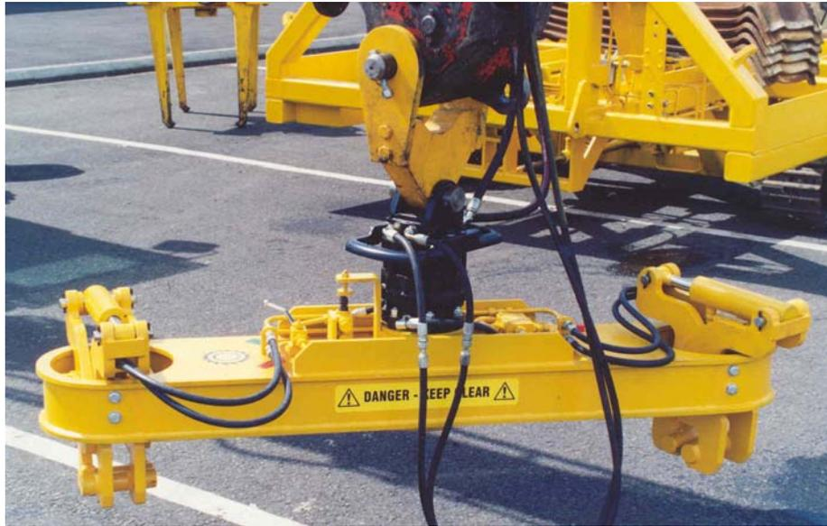
Ensure that the beam is resting on firm, level ground and attach the adapter head to the excavator boom by the attachment head pin.
