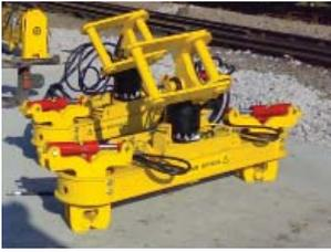
We were approached by a customer who wanted to have the hydraulic rotator on one of his Universal Lifting Beams replaced with a low profile head for attachment to a swivel hook.
