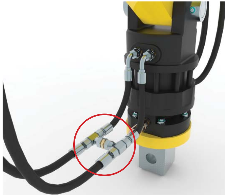
Rotator hoses are connected together using a 1mm bore fitting to dampen out shock loadings
