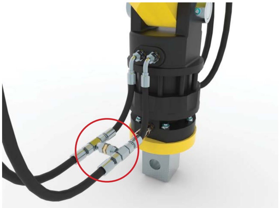
Rotator hoses are connected together using a 1mm bore fitting to dampen out shock loadings
