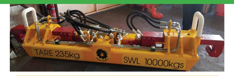
OUR LOW HEADROOM BEAM places the suspension point just above the rail head height allowing more panels to be stacked on wagons when working under overhead electrical installations
