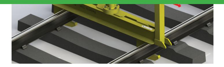
HOOK LIFTING BEAMS are designed for tandem lifting of track panels using any crane type.
