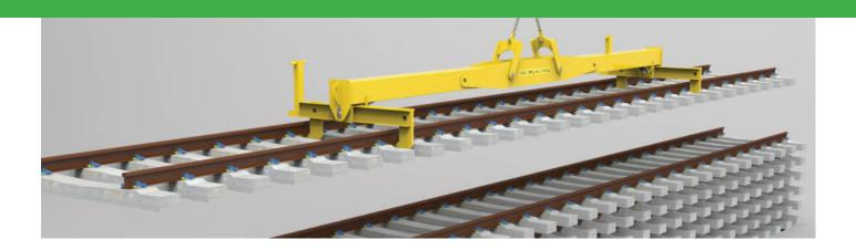
THE CPB20-01 PANEL HANDLER combines the simplicity of our HOOK LIFT BEAMS with a rigid central beam, significantly reducing the headroom requirement when lifting track panels with cranes.
