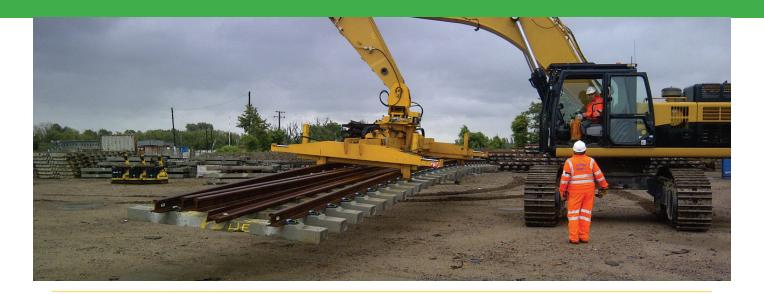
THE MEGABEAM SYSTEM is a suite of products designed for loading and unloading rail components onto works trains. The system comprises the Megabeam, a custom designed rotator / adapter system and various other attachments for handling rails, rail bundles, sleepers and general goods.
