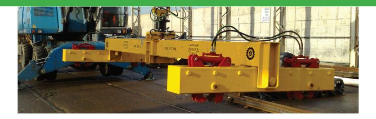
THE PH16-02 PANEL HANDLER is a heavy-duty single lift panel beam designed for full-time usage in rail handling yards.
