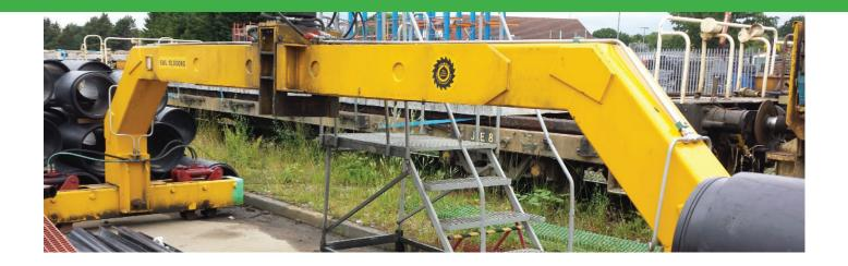
THE PH16-03 uses the same grab system as the PH16-02 but features an arched centre beam making it more stable when lifting long panels.
