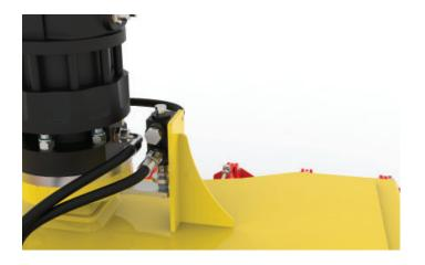
A pressure control valve ensures that the device may be used with almost any machine.
