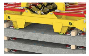
All parts of the device which come into contact with the concrete surfaces of the sleepers are fitted with urethane pads to prevent damage to the sleeper surfaces
