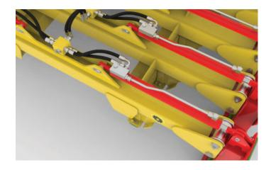
For extra safety, steel toe plates on the jaws pass beneath the sleeper ends.  $\label{eq:pass}$
