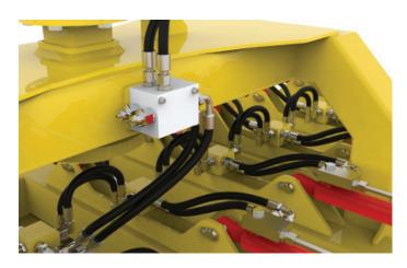
Every hydraulic cylinder is fitted with a pilot-operated check valve to automatically lock the cylinder in the event of a hose burst or other hydraulic failure.
