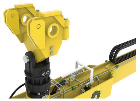
A custom built adapter head may be supplied to suit any host machine. The clamshell type head shown is suitable for Fuchs machines and is mounted on the hydraulic rotator. The white handle near the rotator is used to extend and retract the telescopig ends of the beam.
