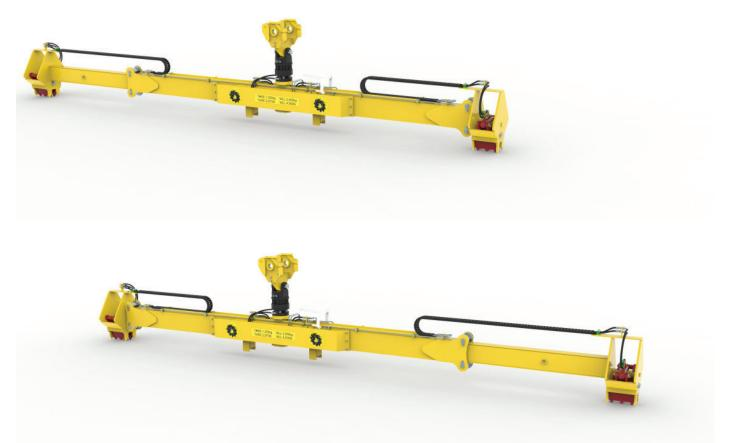
Unless the white handle is depressed the hydraulic supply to the jaws is diverted to the telescopic loadlevelling function when the beam is lifted. In this way the beam can 'side shift' to aid the handling of long rail sections.
