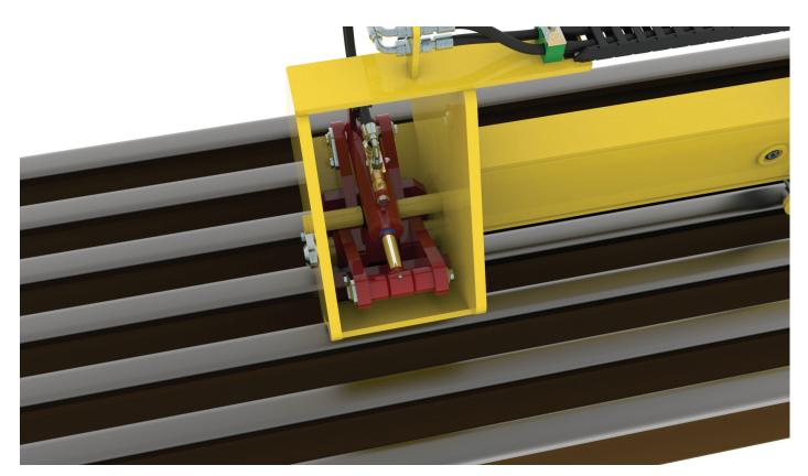
Heavy-duty jaws gripping the rail. The jaws are designed to fit between the heads of tightly bundled rails.
