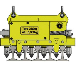
To lock safely into the rails, the spacing of the locking shafts of the rail handler must match the width of the rail foot. On MRH14 units the spacing is fixed, on MRL18 units the spacing is adjustable.
