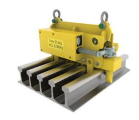
Hydraulically actuated MRH14 units have a pilot operated check valve on the cylinder to lock the mechanism in the event of a burst hose or other hydraulic system failure.
