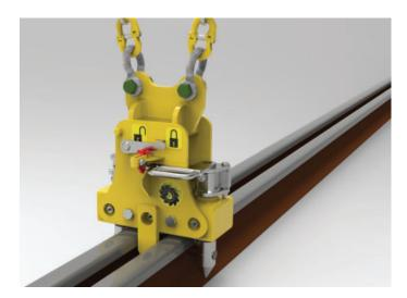
Electrically operated MRH14 Rail Handlers use a 24V DC motor driving a screw actuator to open and close the mechanism.
