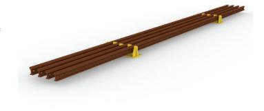
When the base rack layer has been filled with rails, layer racks are place on top of the rails close to the base racks.
