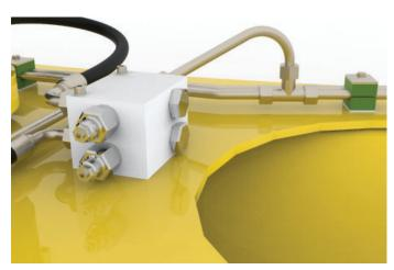
The 'parachute valve' mounted close to the rotator automatically shuts off the connection to the host machine hydraulic supply once the device is lifted.
