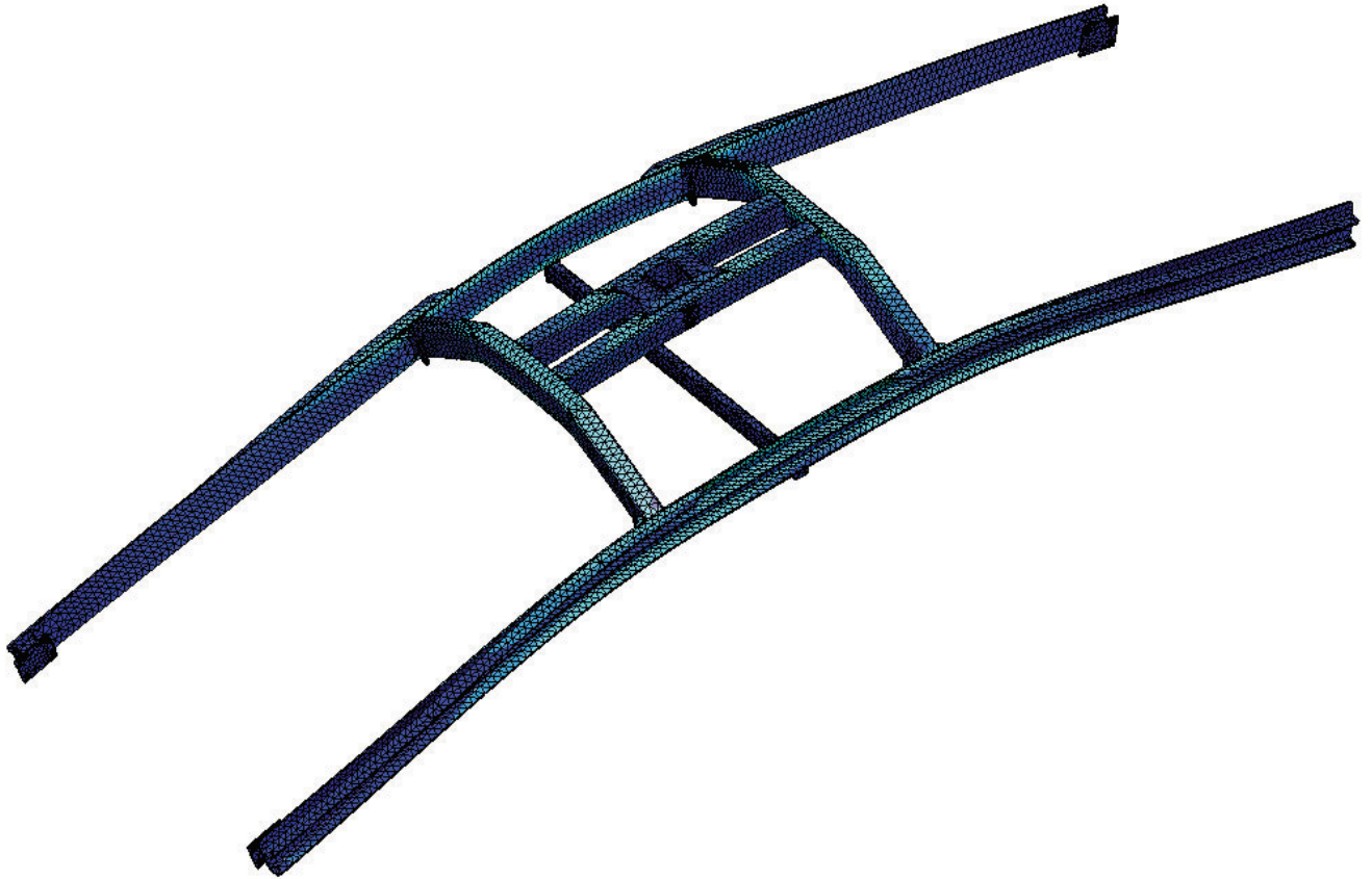
Computerised stress analysis of the chassis
